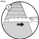
STEP 3. When it is sticking out the side, pull it out in the same direction with a pair pliers, like you would a tooth. Scrape or file the nut slot free from old glue and finish residue while making sure that slot remains square.
