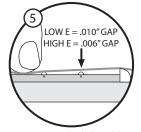
STEP 5. Restring the high and low E strings and tune to pitch to check for correct height. Pushing down on the third note of the low E string should result in a .010" gap between the string and the first fret; high E string should be no6"
