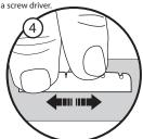
STEP 4. See if the Graph Tech nut fits into the slot, without forcing it. If it's too thick, place a 400 to 600 grit sand paper face up on a flat surface and sand down the sides of the nut until it fits in the slot snugly but is easily removable.
